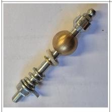
BR Mk1 Passenger door hinge pin assembly.
