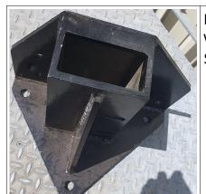
BR Mk1 Vestibule Buffer Stem Bracket. Steel fabrication.
